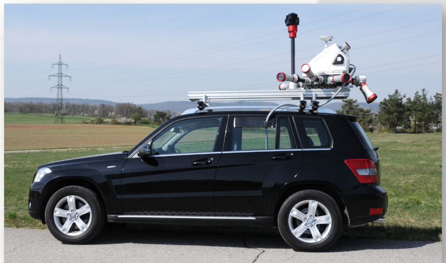
RIEGL VMX-2HA system mounted by means of the VMX-2RM Reinforced Roof Mount
